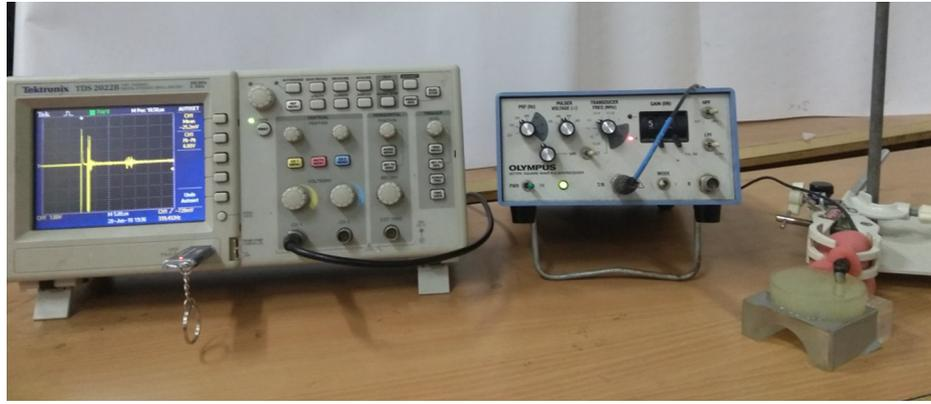
Fig. 4. A photo of the experimental setup used for measuring and characterizing the acoustic properties of the test samples.
