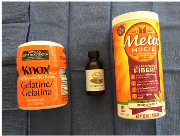
Figure 1 This photo displays the core ingredients used to make ballistics gel for several of the displayed simulation phantoms (powdered “Knox” gelatin, cinnamon leaf oil and “Metamucil” fiber).
