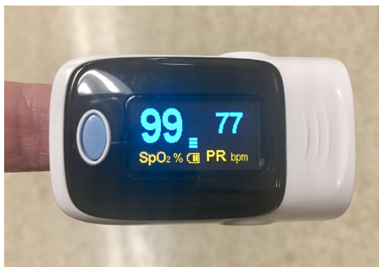
Figure 1 Battery operated, portable pulse oximeter that can be easily used in a clinic setting.
