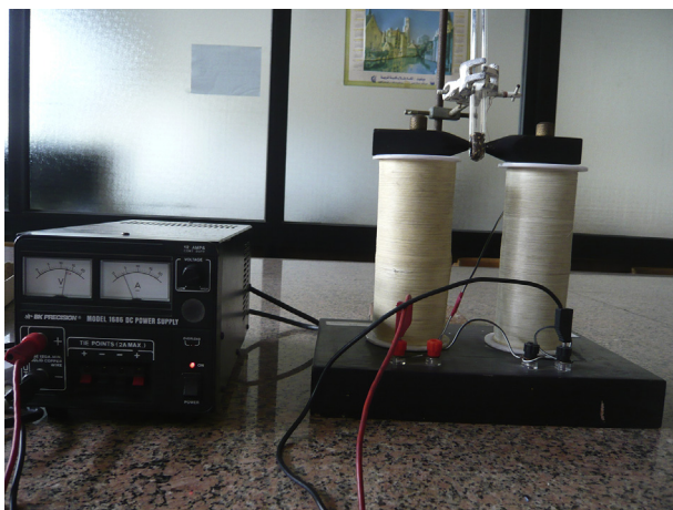
Fig. 2. Magnetic susceptibility device (0.18 T).
