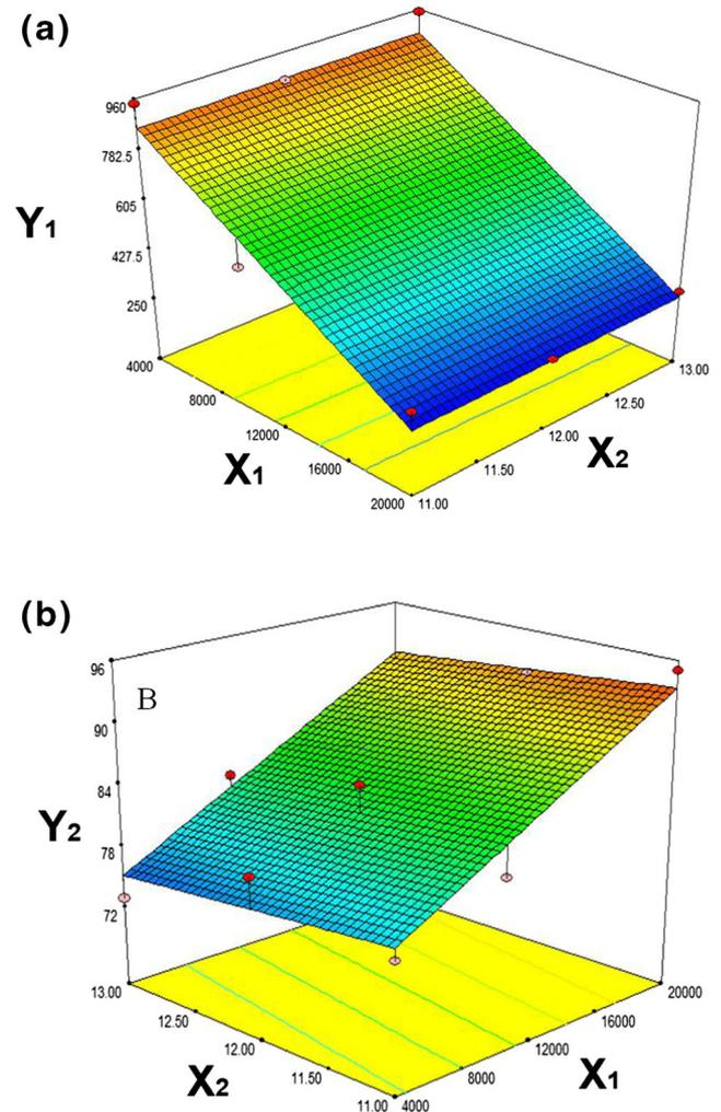
**Fig. 3** Three-dimensional surface response plot showing the effect of polymer molecular weight and drug polymer ratio on the particle size (a) and entrapment efficiency (b). X<sub>1</sub>, molecular weight of PEG; X<sub>2</sub>, drug polymer ratio; Y<sub>1</sub>, mean particle size (nm); Y<sub>2</sub>, entrapment efficiency (%)
