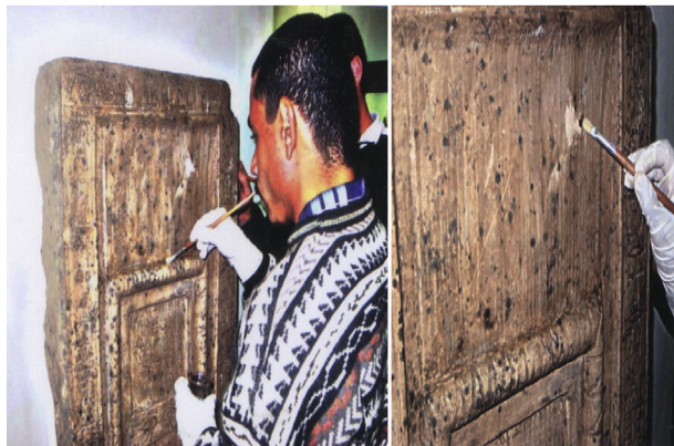
Fig. 7. p -chloro- m -crysol at concentration 50 ppm applying for False-door. Treatment by brush method.
