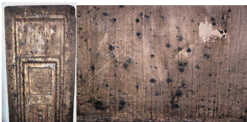
Fig. 1. Fungal infection on limestone (Black spots) of False-door.
