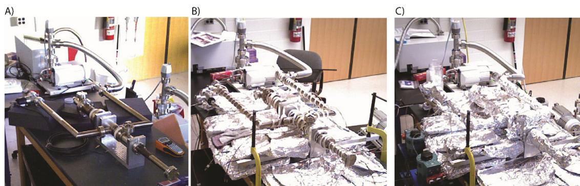
Fig. 10. Gyrotron bakeout. (A) Assembled gyrotron connecting to a turbomolecular pump. (B) Gyrotron wrapped with heating tapes. Thermocouples are placed in different regions to monitor temperatures. (C) The gyrotron is further wrapped in aluminum foil to trap heat.
