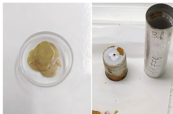
Fig. 10. Left: Krytox 240 AC sample irradiated at 0.97 MGy (3 h and 30 min). Right: the aluminum set-up used for irradiation. The stopper has been corroded by the acid gases evolved.
