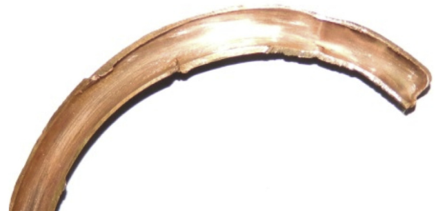
Fig. 11. Assessment of deposit of MWCNTs on coiled tube before conducting tests.
