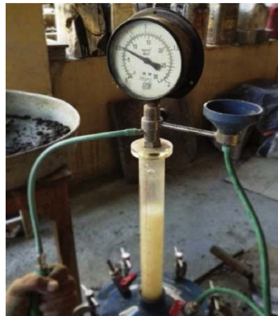
Fig. 1. Setup for air entrainment of fresh concrete test.
