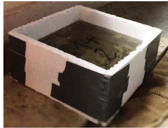
Fig. 3. Configuration of the concrete slab during the ponding.
