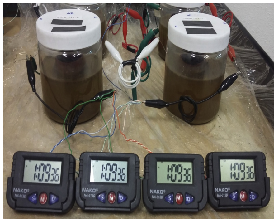
Fig. 5. Both-C-MFCs connected in series in order to power the digital clocks.
