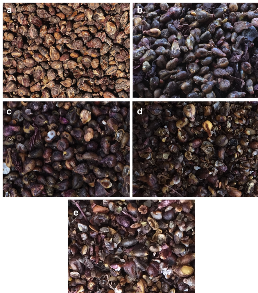
Fig. 7. Comparison of seeds of the control (a) and the seeds obtained by Type- B blade settings at: b) 480 rpm; c) 576 rpm; d) 672 rpm; e) 864 rpm.
