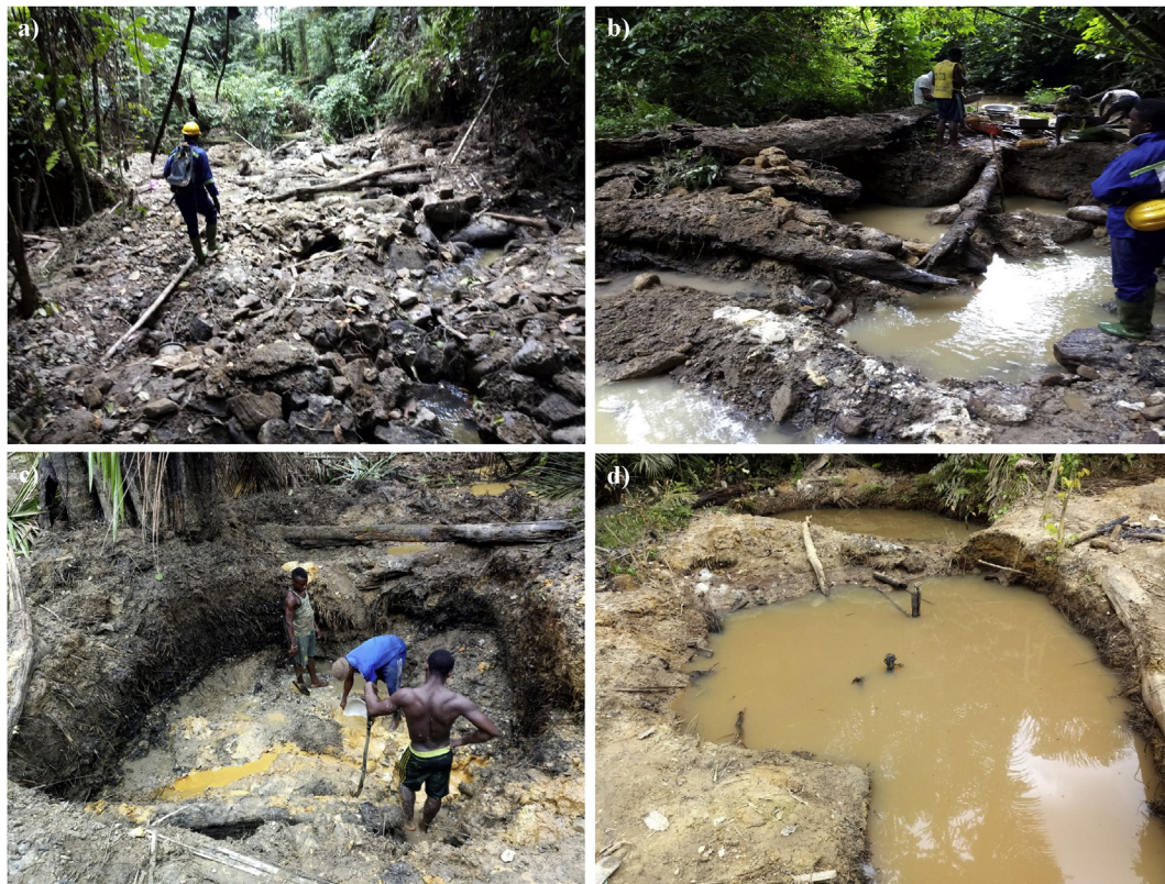
Fig. 6. The physical degradation of ecosystems: a) destruction of the forest ecosystem; b) relocation of stream beds; c) land section with rectangular shape and d) geometric forms according to the layout of the mining grounds.
