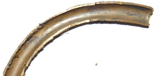
Fig. 17. After test surface of coil inner surface.
