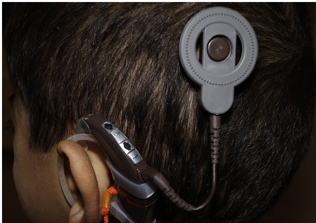
Figure 1 After the reversal of the external magnet, the external part appears to hold on to the internal part.
