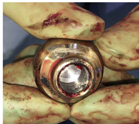
Figure 5. Metal head with fretting corrosion seen within the bore.
