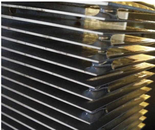
Fig. 16. Tilted heatsink condensate bridging at 60°.
