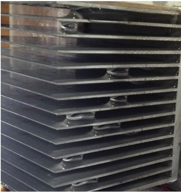
Fig. 11. Rotated heatsink at 45° angle.
