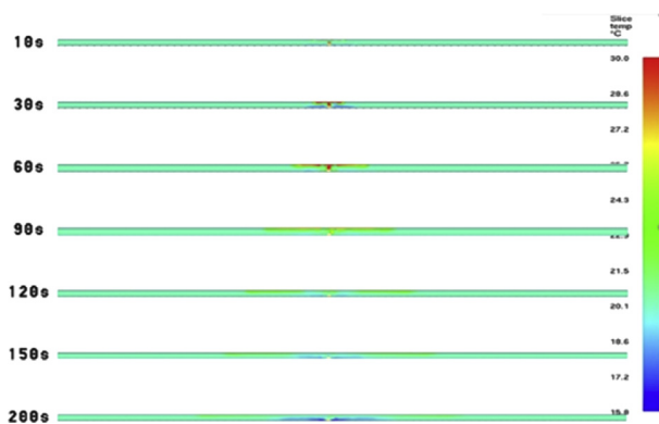
Fig. 18. Temperature contour at 2 m above the tunnel floor in the presence of the basic water mist system.
