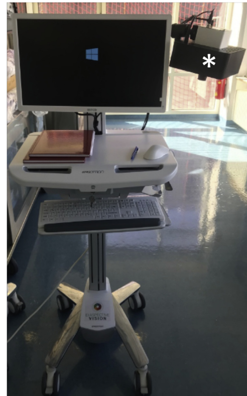
Fig. 2. TIVITA® device with light source and HSI camera (*). The chemical color imaging procedure is calculated with the attached computer.
