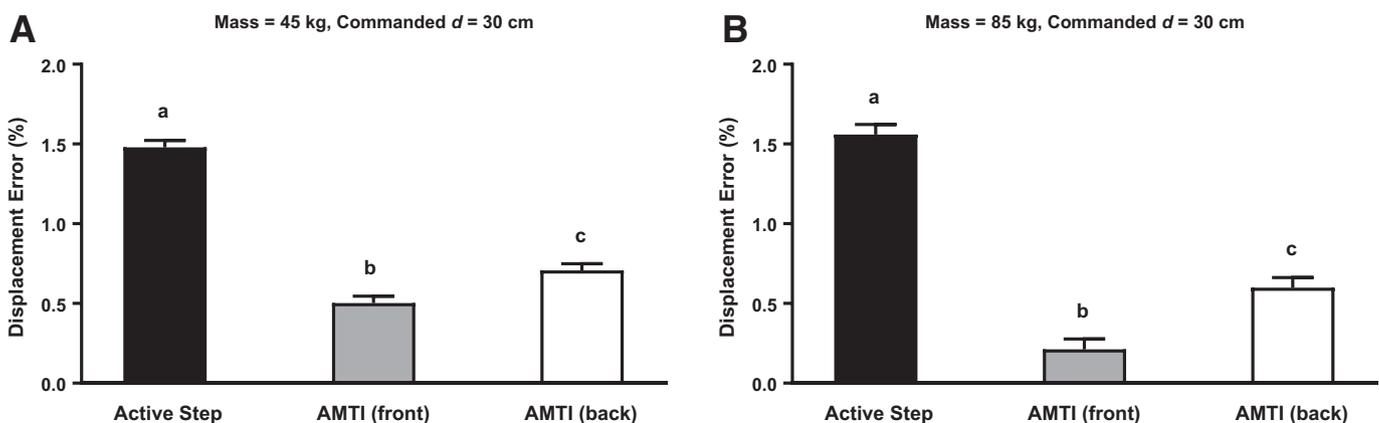
**Fig. 2.** Estimated marginal means (standard errors) of relative errors (observed – commanded / commanded) in total displacement, estimated at a commanded displacement of 30 cm and bearing masses of 45 kg (A) and 85 kg (B). Significant ( $p < 0.01$ ) between-treadmill-belt differences are noted with different letter labels (a, b, c).
