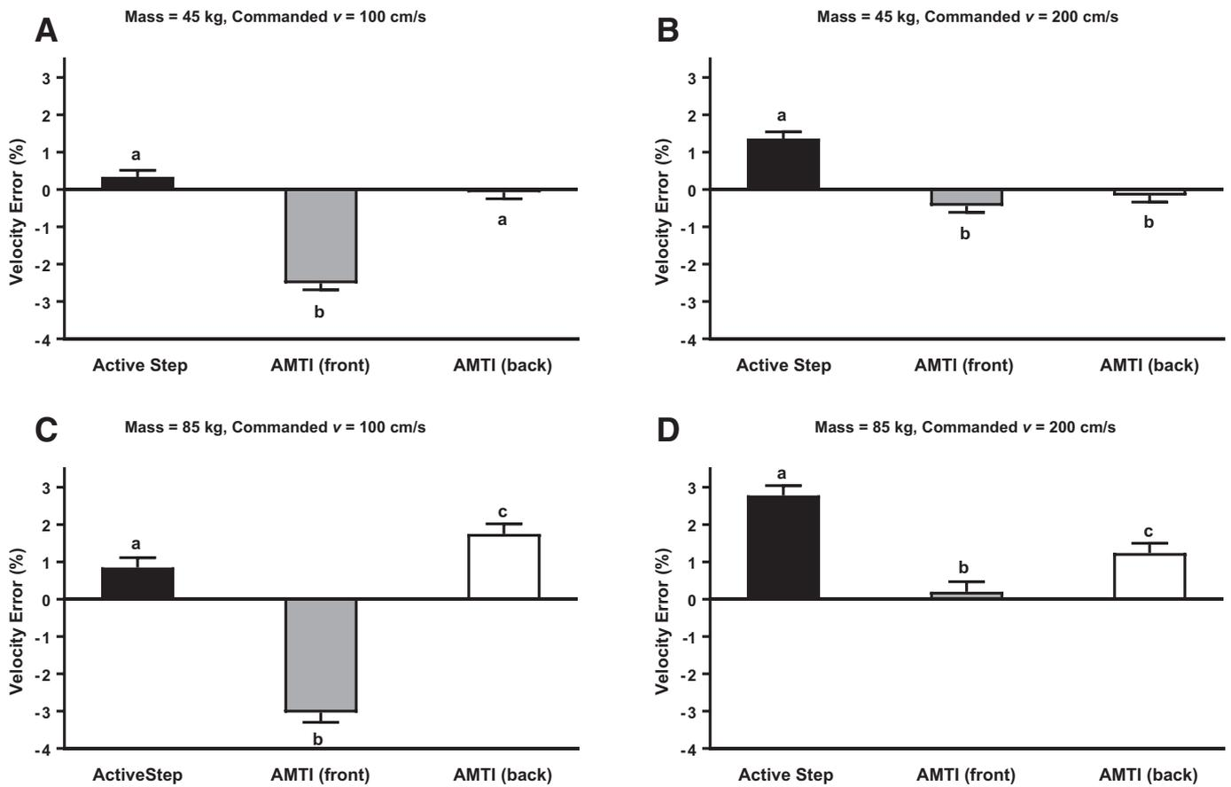
**Fig. 3.** Estimated marginal means (standard errors) of relative errors (observed – commanded / commanded) in peak velocity, estimated at commanded velocities of 100 cm/s (A & C) or 200 cm/s (B & D), as well as bearing masses of 45 kg (A & B) or 85 kg (C & D). Significant ( $p < 0.05$ ) between-treadmill-belt differences are noted with different letter labels (a, b, c).
