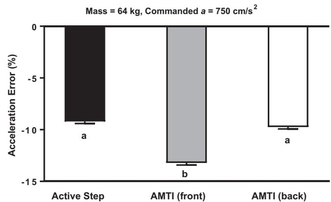
**Fig. 4.** Estimated marginal means (standard errors) of relative errors (observed – commanded / commanded) in initial average acceleration, estimated at a commanded acceleration of 750  $\text{cm/s}^2$  bearing a mass of 64 kg. Significant ( $p < 0.001$ ) between-treadmill-belt differences are noted with different letter labels (a, b, c).
