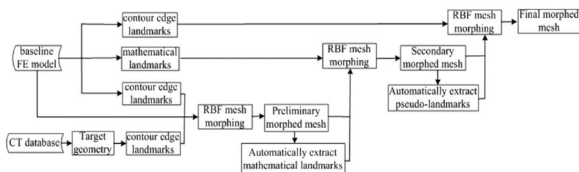
**Figure 2.** Procedure to develop the target FE mesh.
