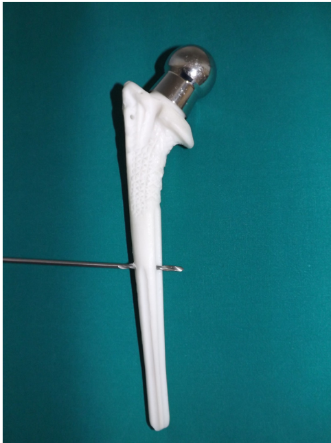
Fig. 3. The femoral component of the third-generation isoelastic RM® total hip replacement is easily perforated with a 3.2 mm drill due to their polymeric composition.
