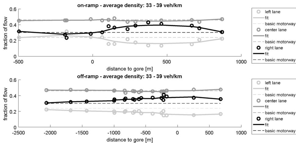
Fig. 6. Lane flow distribution at ramps.
