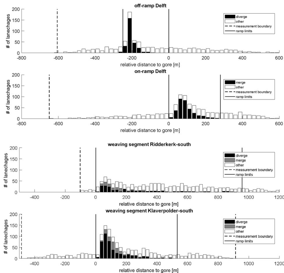
Fig. 4. Lane change locations near on-ramps and off-ramps.
