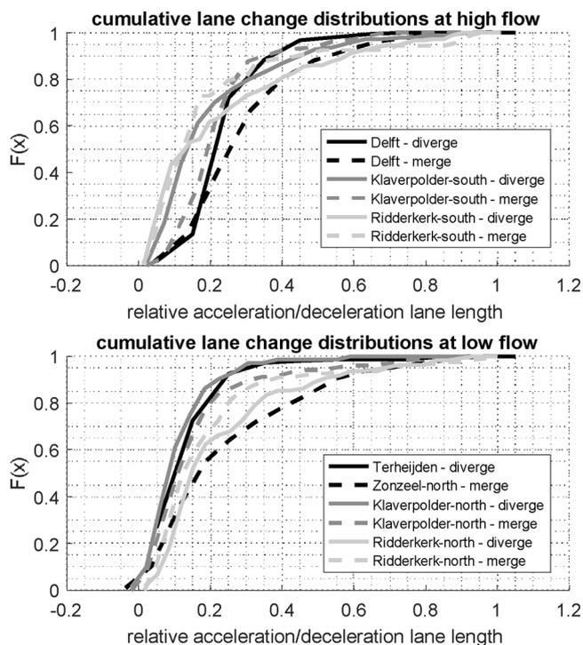
Fig. 5. Use of acceleration and deceleration lane under different conditions.
