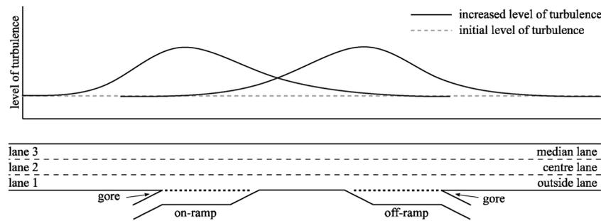
Fig. 1. Concept of the level of turbulence around succeeding ramps.
