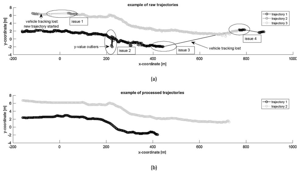
Fig. 2. Example of raw (a) and processed trajectories (b).
