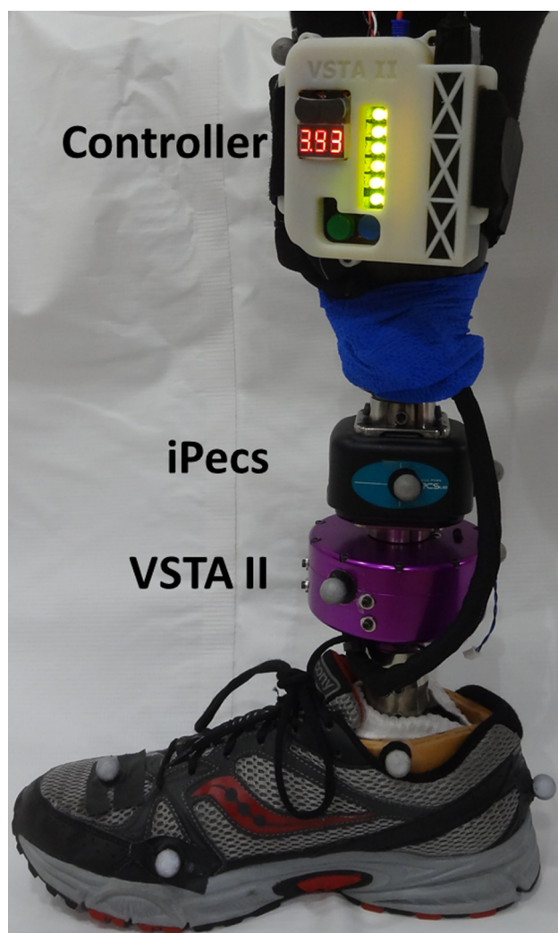
Fig. 1. VSTA II instrumentation. System included a standalone controller with on-board battery, an iPecs 6-axis load cell to measure limb loading at the socket interface and the VSTA II device attached to the shank of the lower-limb prosthesis.
