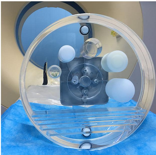
**Fig. 2** Vitro pancreatic stone was placed into a TOS water phantom, with 35 cm lateral width
