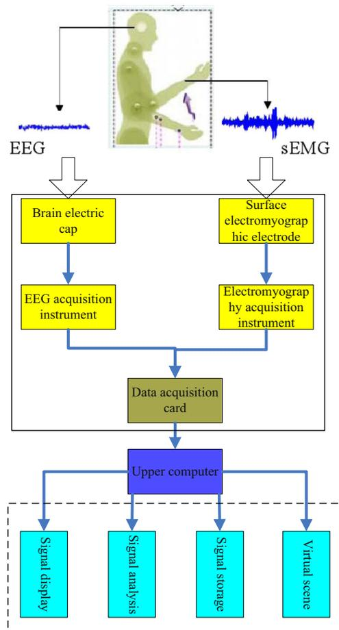
Fig. 2 Block diagram of EEG signal acquisition system
