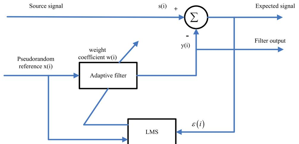
**Fig. 4** Removal of power frequency interference by adaptive filter
