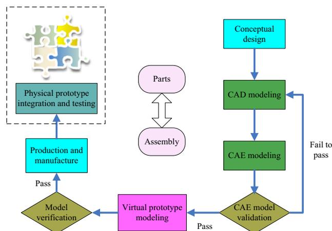
Fig. 1 Flow chart of virtual prototype modelling
