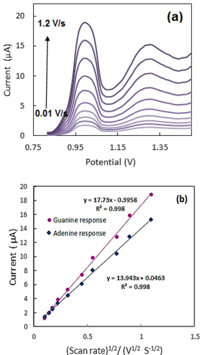
**Fig. 9.** (a) DPV voltammograms of CPE/MWCNT/Ag NPs/ds-DNA MIS in 0.5 M acetate buffer (pH 4.8) containing 40 μmol L<sup>-1</sup> of GEM in potential scan rate of 0.01–1.2 V/s, and (b) obtained plots of anodic peak current vs. square root of potential scan rate for GEM based on the change of oxidation response of guanine and adenine.
