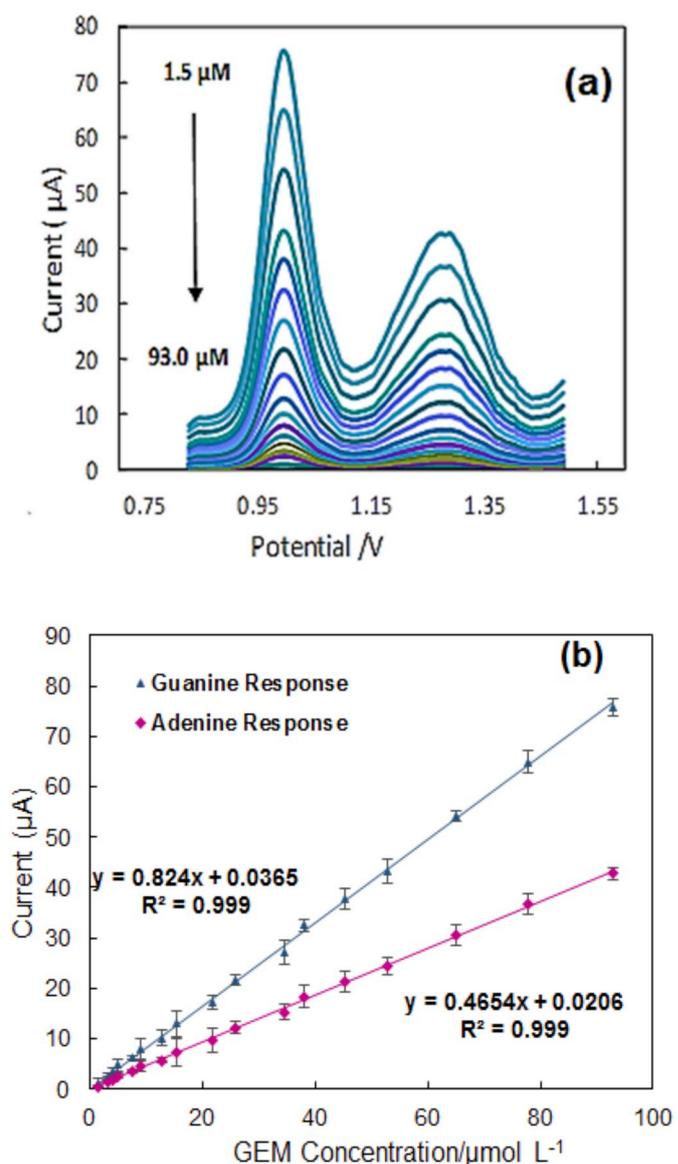
**Fig. 8.** (a) DPV voltammograms of CPE/MWCNT/Ag NPs/ds-DNA MIS in 0.5 M acetate buffer (pH 4.8) upon increasing the concentration of GEM in the range of  $1.5 \text{ } \mu\text{M}$ – $93 \text{ } \mu\text{M}$  under optimized condition, and (b) and its corresponding calibration curves for GEM based on the change of oxidation response of guanine and adenine.
