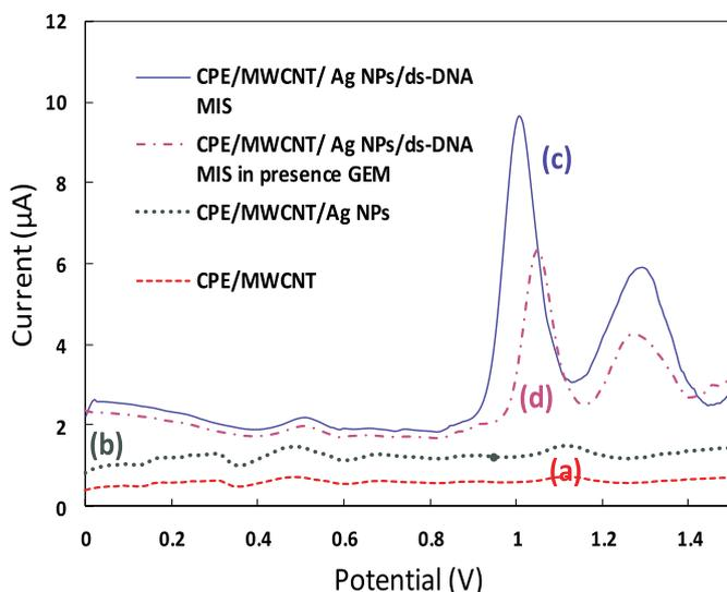
**Fig. 7.** DPV voltammograms of CPE/MWCNT (curve a), CPE/MWCNT/Ag NPs (curve b), CPE/MWCNT/Ag NPs/ds-DNA MIS film in absence GEM (curve c) and CPE/MWCNT/Ag NPs/ds-DNA MIS film in presence of GEM (curve d) in 0.5 M acetate buffer (pH 4.8).
