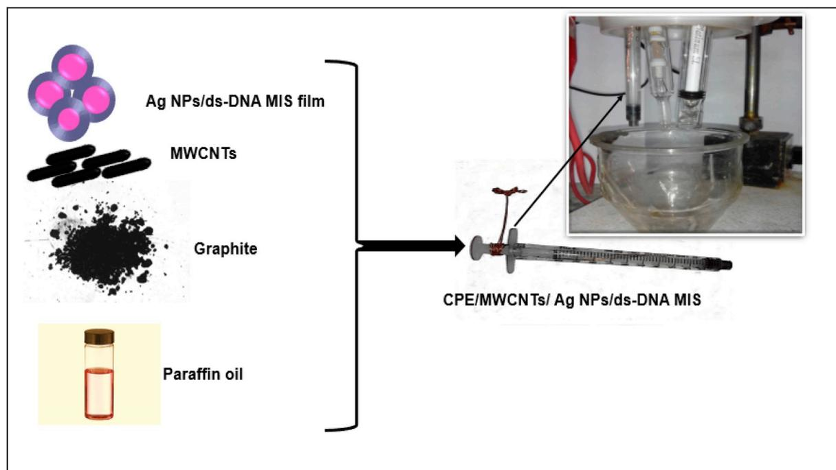
**Scheme 3.** Schematic fabrication of CPE/MWCNTs/Ag NPs/ds-DNA MIS.
