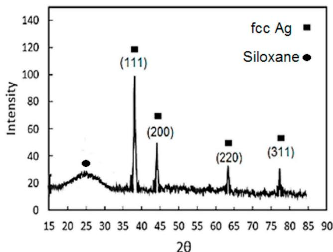
Fig. 3. XRD pattern of the siloxane @ Ag NPs.
