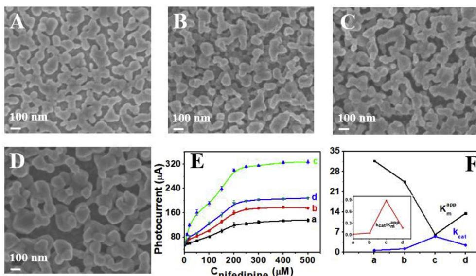
Fig. 4. SEM images of single-layer CuO films (A) and multi-layer CuO films prepared with molar ratio of Cu<sup>2+</sup> and PVP of 5:1 (B), 5:2 (C), or 5:3 (D). (E) Corresponding Michaelis–Menten plots, and (F) kinetic parameters of ITO/CuO/CYP3A4 with single layer (a), and molar ratio of Cu<sup>2+</sup> and PVP of 5:1 (b), 5:2 (c), or 5:3 (d), respectively.
