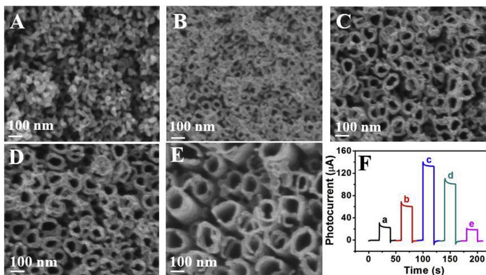
Fig. 3. SEM images (A–E) of TNA/g-C<sub>3</sub>N<sub>4</sub> with 4 h of anodization time and different anodization potentials of 10 V (A), 15 V (B), 20 V (C), 25 V (D) and 30 V (E). (F) Corresponding photocurrent responses of TNA/g-C<sub>3</sub>N<sub>4</sub> with different anodization potentials of 10 V (a), 15 V (b), 20 V (c), 25 V (d) and 30 V (e).
