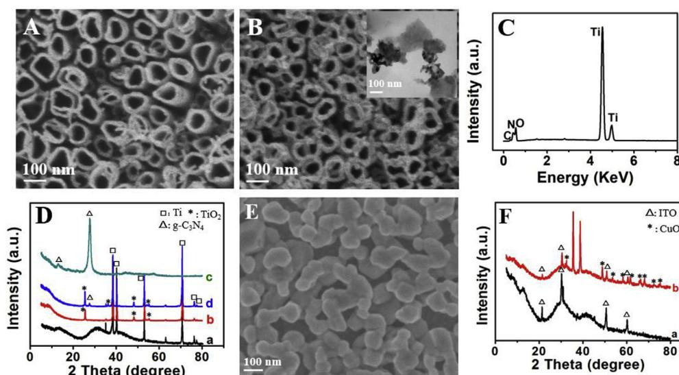
Fig. 1. SEM image of TNA (A) and TNA/g-C<sub>3</sub>N<sub>4</sub> (B), Inset: TEM image of g-C<sub>3</sub>N<sub>4</sub>. (C) EDS of TNA/g-C<sub>3</sub>N<sub>4</sub>. (D) XRD pattern of Ti substrate (a), TNA (b), g-C<sub>3</sub>N<sub>4</sub> (c) and TNA/g-C<sub>3</sub>N<sub>4</sub> (d). (E) SEM image of ITO/CuO. (F) XRD patterns of ITO (a) and ITO/CuO (b).
