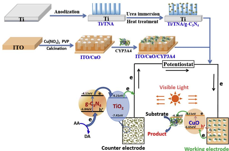
**Scheme 1.** Construction of the double photoelectrode system for photoelectrochemically driven enzymatic bioconversion and determination of target.
