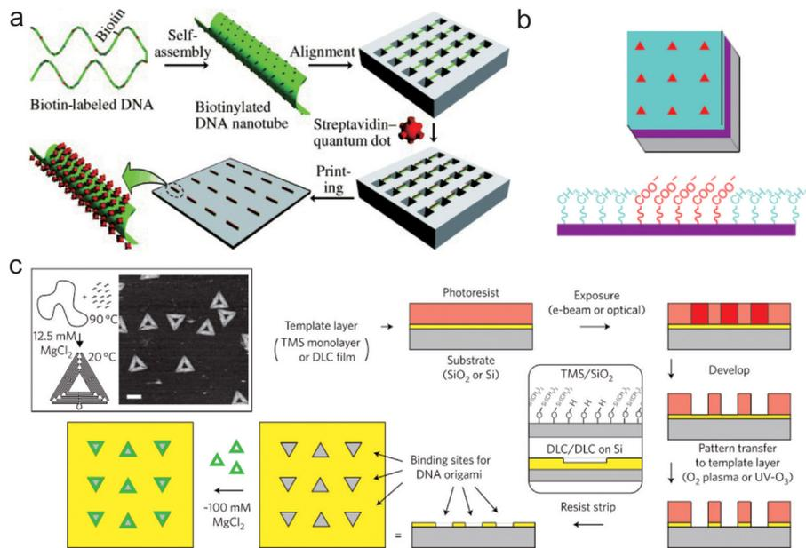
**Fig. 14.** DNA lithography with noncovalent interactions. a) Alignment of DNA nanotube arrays. Reprinted with permission from ref. [130] Copyright © 2007, John Wiley and Sons. b) Fabrication of a single binding site for DNA origami mediated by cationic ions. Reprinted with permission from ref [132], Copyright © 2016, Springer Nature. c) Placement of individual DNA origami through hydrophilic interactions. Reprinted with permission from ref [133], Copyright © 2009, Springer Nature.
