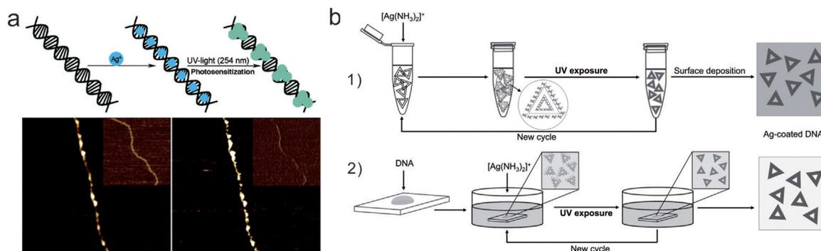
**Fig. 9.** DNA metallization through photochemical reduction. a) Photoinduced silver deposition on DNA templates. Reprinted with permission from ref. [100] Copyright © 2005, American Chemical Society. b) Photochemical reduction for silver coating of DNA origami using (1) solution route or (2) surface route. Reprinted with permission from ref [102]. Copyright © 2018, IOP Publishing.
