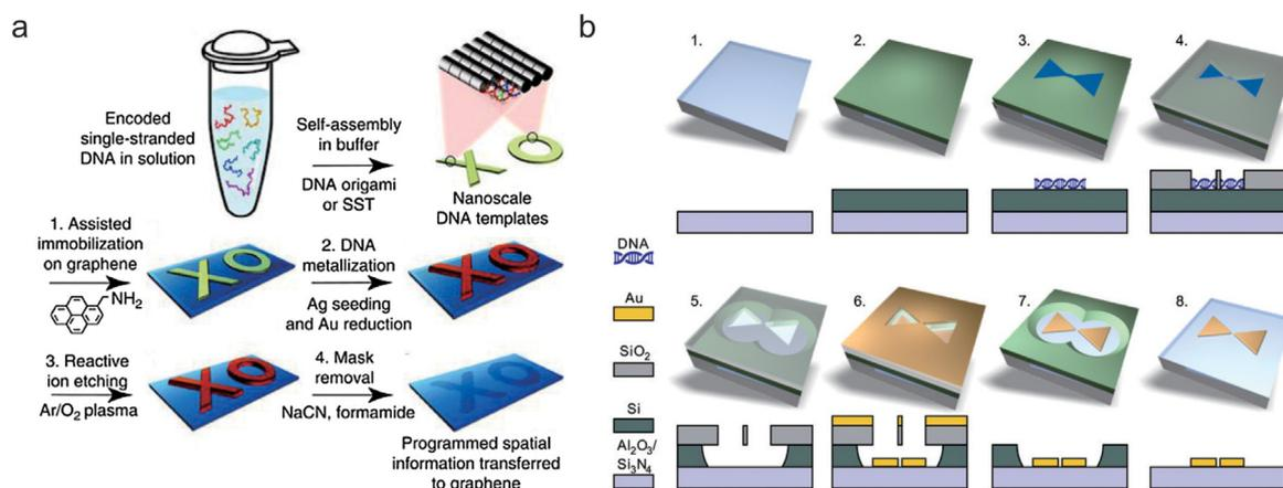
**Fig. 13.** Pattern transfer with Plasma etching. a) Metallized DNA nanostructures as plasma etching resist for graphene nanopatterning. Reprinted with permission from ref. [128] Copyright © 2013, Springer Nature. b) Step-by-step fabrication procedure of the DNA-assisted lithography method. Reprinted with permission from ref [129]. Copyright © 2018, The American Association for the Advancement of Science.
