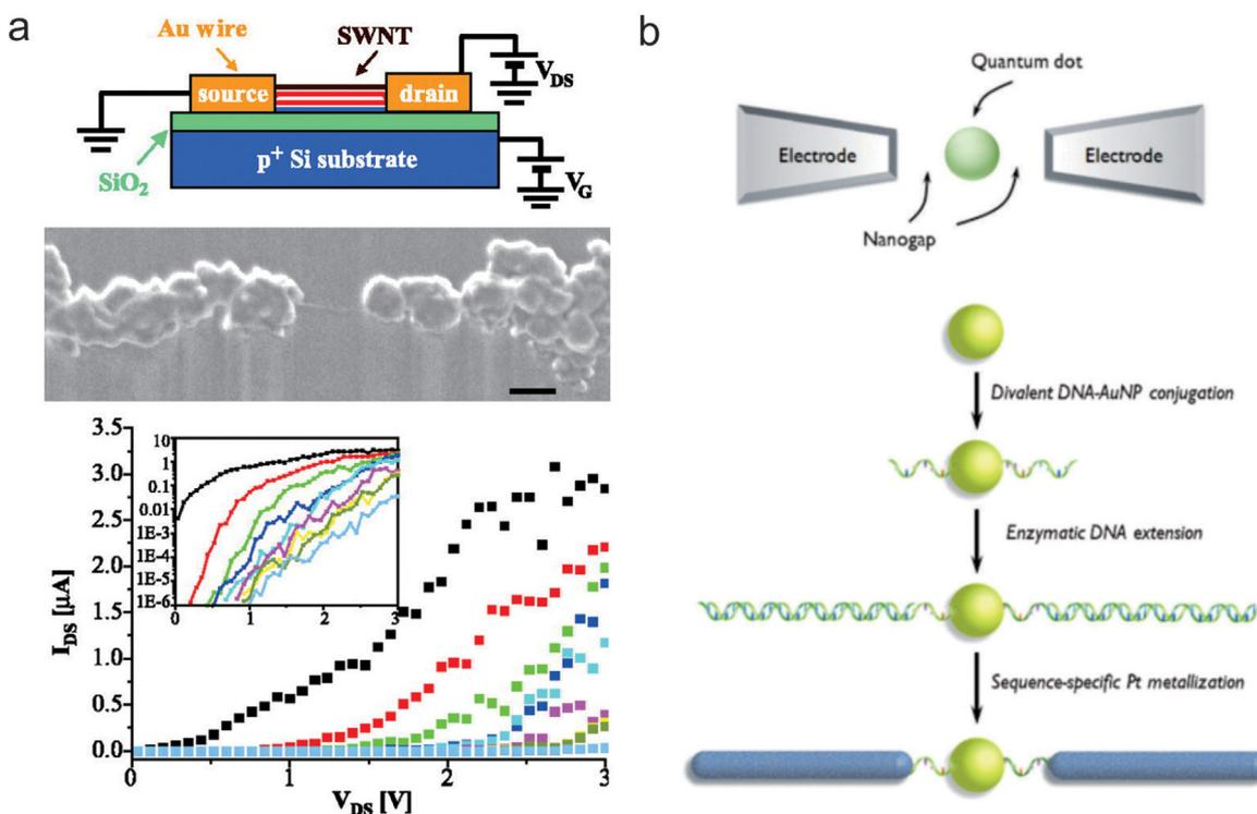
**Fig. 25.** Conducting devices fabricated by DNA metallization. a) Carbon nanotube field-effect transistor based on DNA templated Au metallization. Reprinted with permission from ref. [207] Copyright © 2003, The American Association for the Advancement of Science. b) Fabrication of double tunnel junction single-electron device by Pt metallization of divalent DNA-AuNP conjugates. Reprinted with permission from ref [208]. Copyright © 2012, John Wiley and Sons.
