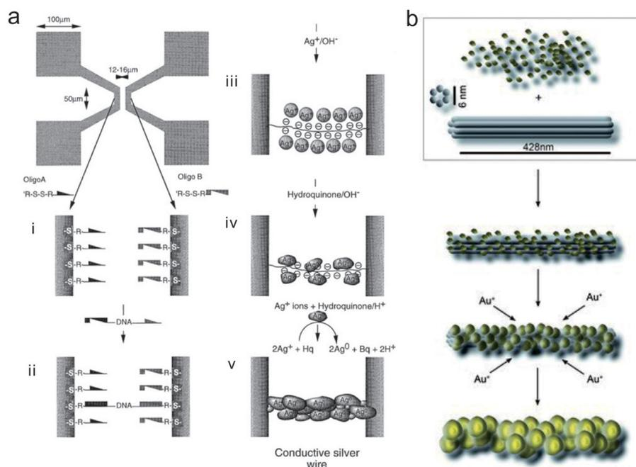
**Fig. 5.** DNA metallization through chemical reduction. a) Constructing a DNA-templated nanowire between two gold electrodes. Reprinted with permission from ref. [71] Copyright © 1998, Springer Nature. b) DNA origami-templated metallization of positively charged nanoparticles. Reprinted with permission from ref [73]. Copyright © 2011, John Wiley and Sons.
