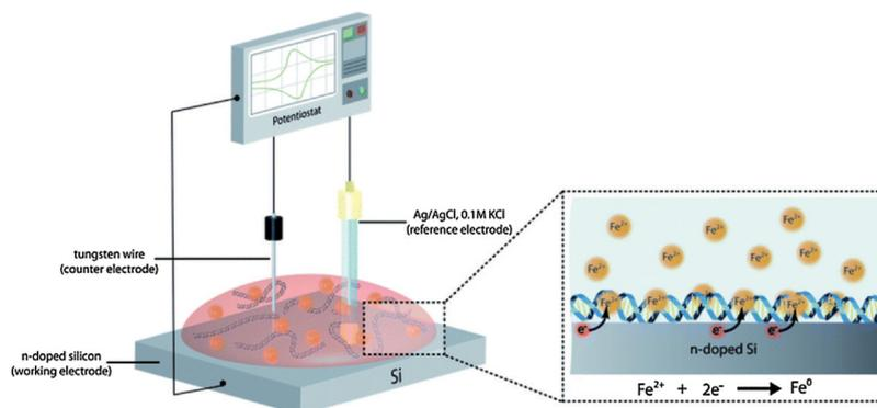
**Fig. 8.** DNA-templated Fe nanowires produced by electrochemical approach. Reprinted with permission from ref. [98] Copyright © 2013, Royal Society of Chemistry.
