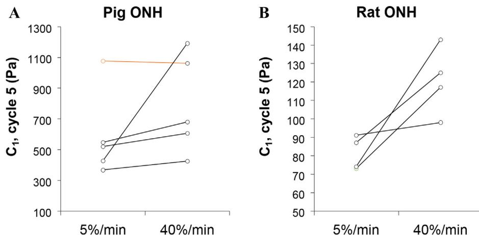
**Fig. 3.**  $C_1$  values for a subset of pig (A) and rat (B) samples that were tested at both 5%/min and 40%/min strain rates. The sample identified as an outlier in the larger porcine 5%/min data set (Fig. 2) is indicated in orange. (For interpretation of the references to colour in this figure legend, the reader is referred to the web version of this article.)
