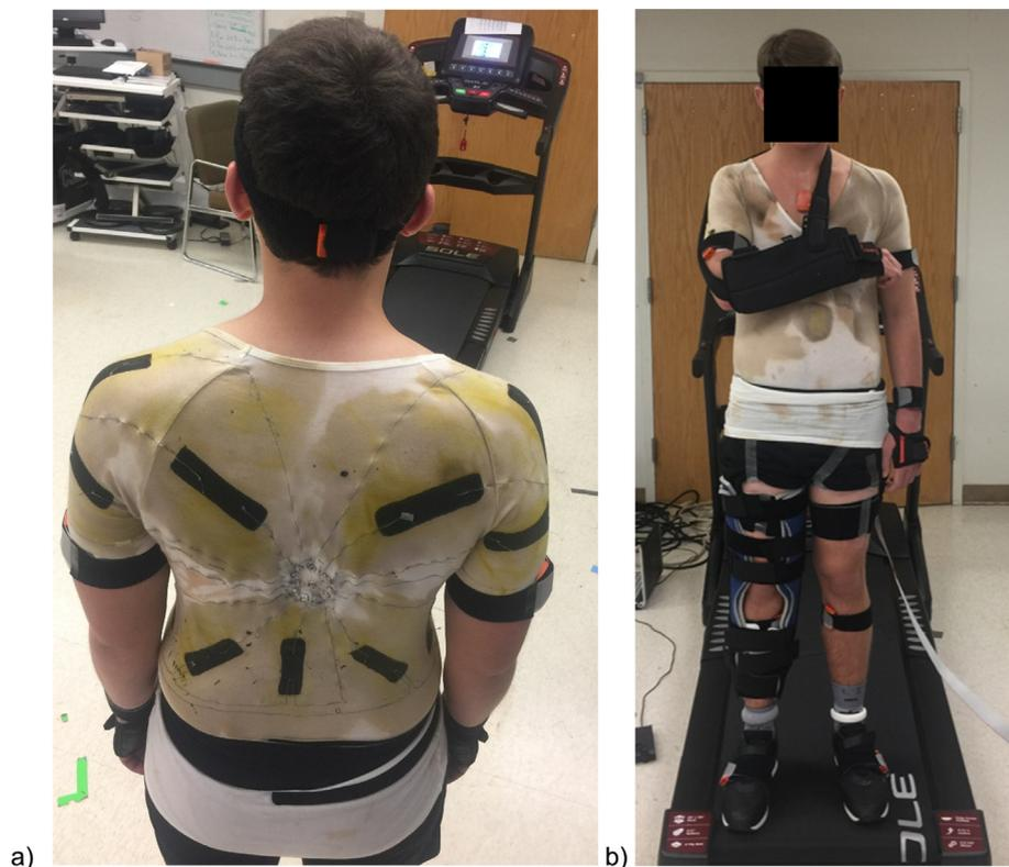
Fig. 2. (a) Illustration of the placement of 11 smart textile sensors on an undershirt (b) An individual wearing both smart garments (smart socks and smart shirt) and unilateral braces on both extremities (for simulating hemiplegic gait).
