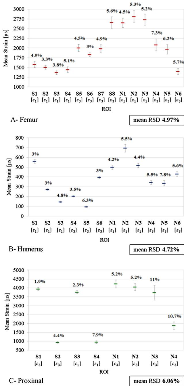
Fig. 5. Mean and RSD values of the maximum absolute principal strains at each ROI across the different scans for the femur (A), humerus (B) and proximal femur (C).
