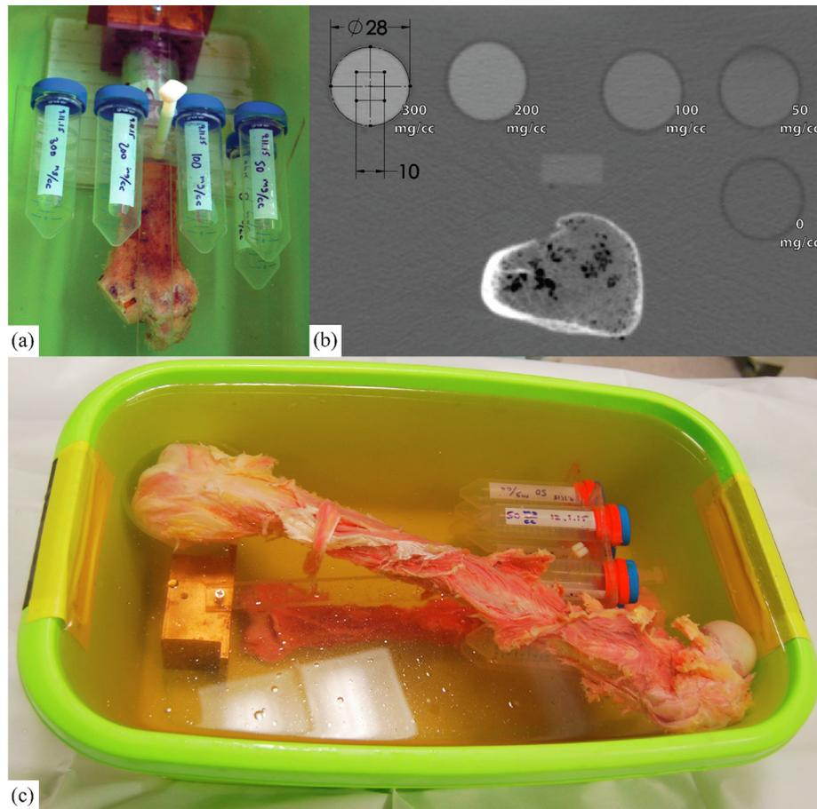
**Fig. 1.** (a) Proximal femur in the water bath surrounded by five liquid potassium phosphate ( $K_2HPO_4$ ) phantoms. (b) A representative CT slice of the femur and phantoms. (c) Whole femur and humerus in water bath with the liquid phantoms.
