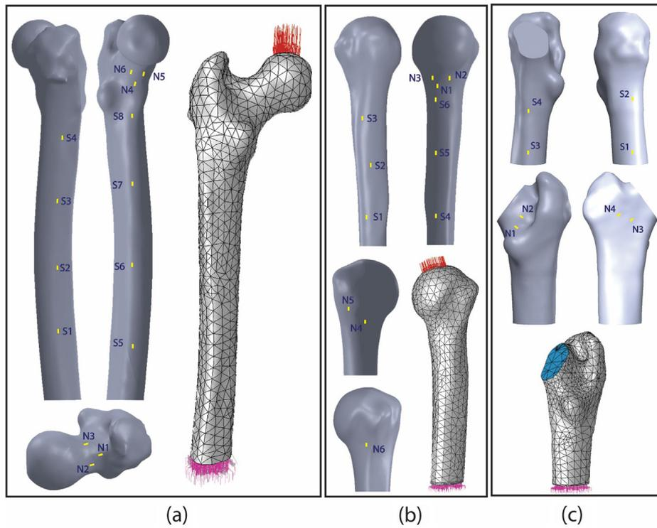
**Fig. 2.** (a) The femur and regions of interest (ROIs) at which strains were extracted with the QCT-based finite element analysis (CTFEA) model and boundary conditions. (b) The humerus and ROIs with CTFEA model and boundary conditions. (c) The proximal femur with ROIs and CTFEA model with displacement boundary conditions.
