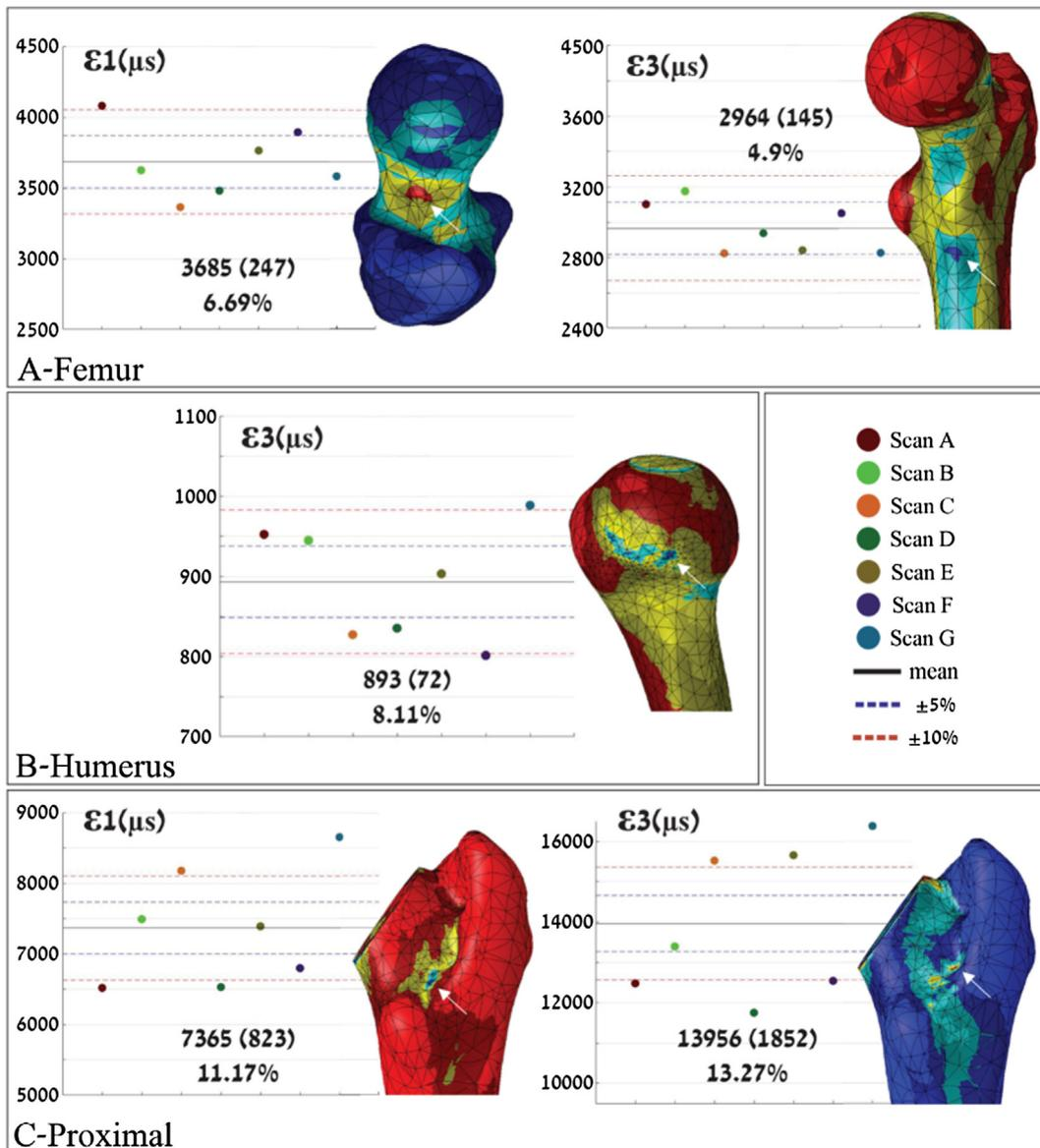
**Fig. 6.** Maximum tensile/compressive ( $\epsilon_1/\epsilon_3$ ) principal strains, in the femur (A), humerus (B), and proximal femur (C). In each panel the mean (SD) and RSD% of the maximal strain is presented. The humerus is under compressive state; thus, no tensile graph is presented.
