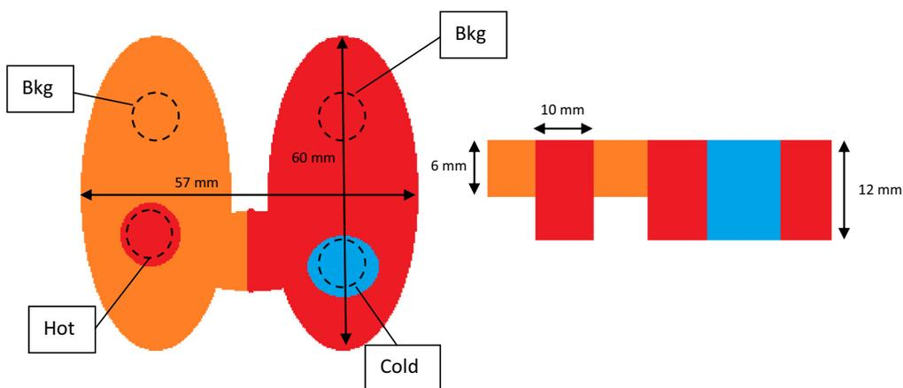
Fig. 2. Schematic of bespoke phantom. Areas in red are twice the depth of the areas in orange. The blue area is solid Perspex and does not contain any activity. (For interpretation of the references to color in this figure legend, the reader is referred to the web version of this article.)
