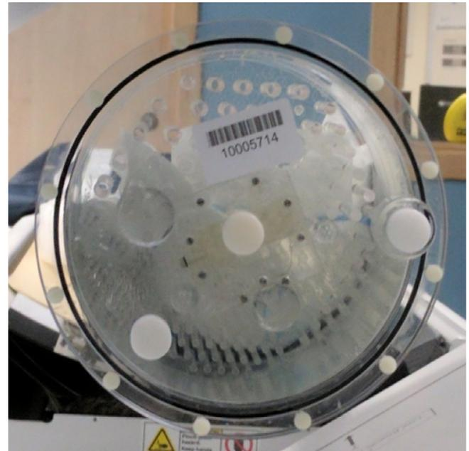
**Fig. 4.** Striatum mimic phantom setup used for SPECT acquisitions.
