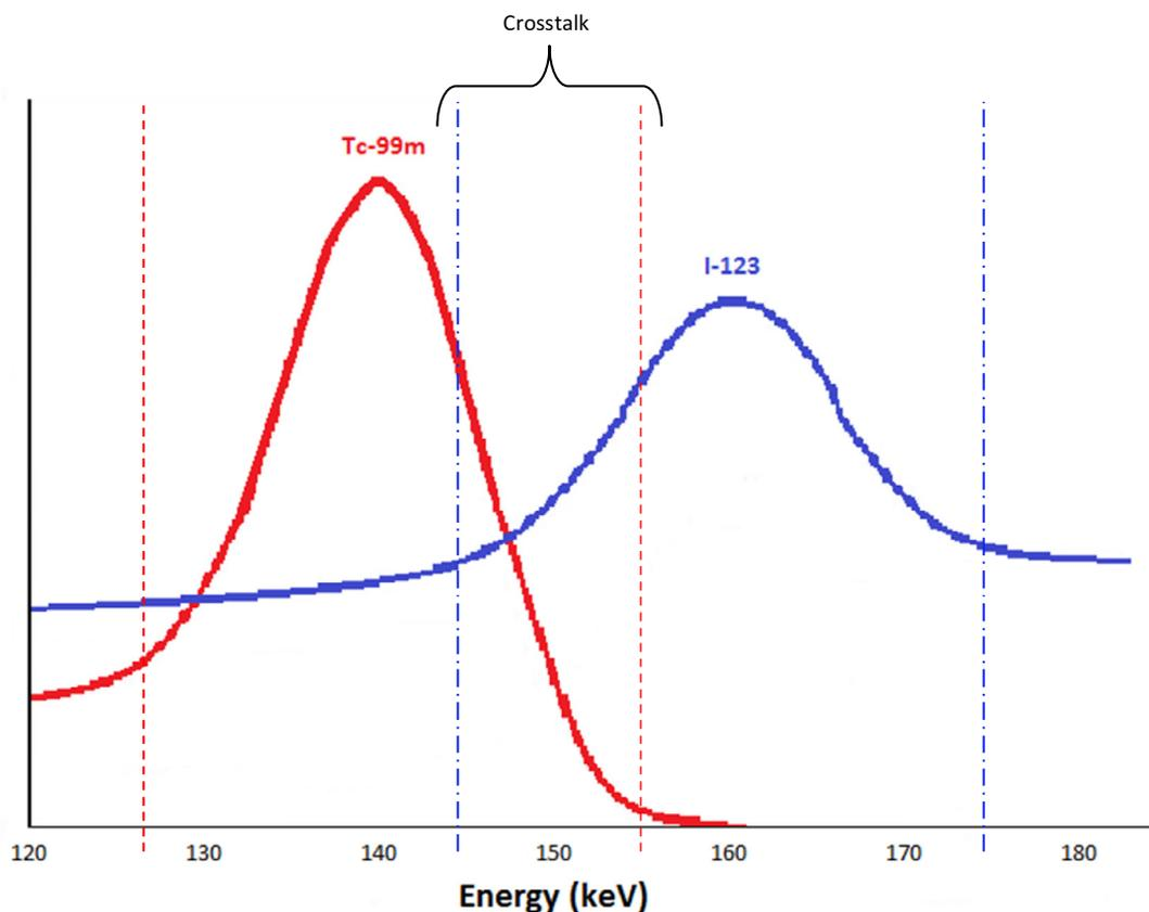
Fig. 1. Energy spectrums of Tc-99m and I-123 gamma photons. Standard energy window boundaries are indicated by dashed lines.
