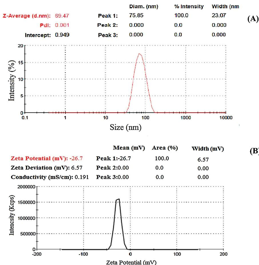
Fig. 6. a) DLS; b) zeta-potential of CUR@[As-PEGylated MSN@GO] nanohybrid.
