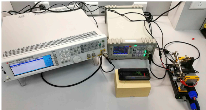
Fig. 17. Our benchtop equipment to carry out the proof of concept reproduction of tones heard in Cuba. Note, we would expect emitters to be smaller than a paperback book in practice, if not smaller. We use large equipment because of our general-purpose laboratory.
