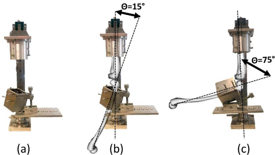
**Fig. 2.** From the left-hand side: (a) the knee alignment rig assembled with the screw mechanism, (b) the first reference configuration (i.e., 15° knee flexion), and (c) the second reference configuration (i.e., 75° knee flexion).
