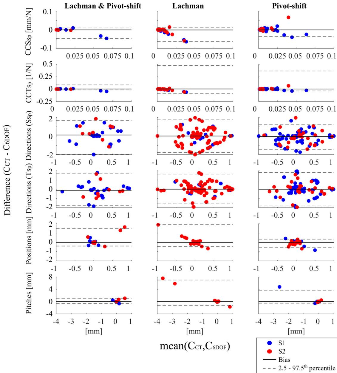
**Fig. 4.** Bland–Altman plot for the comparison of  $C_{CT}$  and  $C_{6DOF}$  principal components (CC: Compliance coefficients;  $S_{Sp}$ : Screw spring;  $T_{Sp}$ : Torsional spring), reporting the 2.5th and 97.5th percentiles as limits of agreement.
