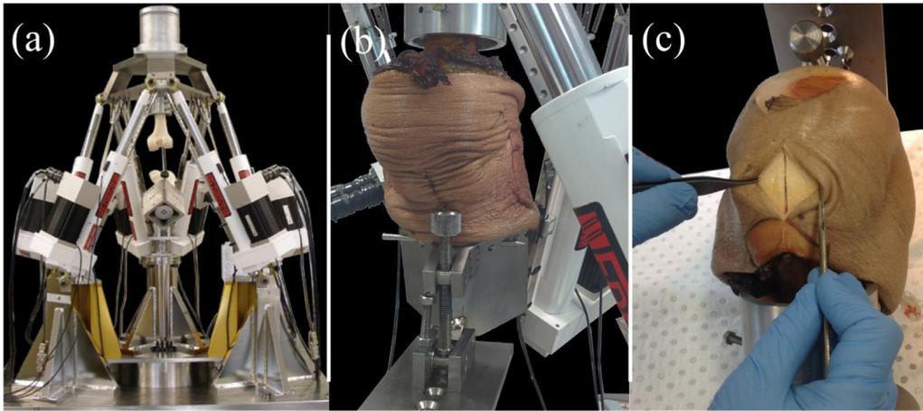
**Fig. 1.** From the left-hand side: (a) frontal view of the hexapod robot and the screw mechanism hosting a dummy femoral and tibial component; (b) detail of one knee specimen mounted on the hexapod robot through the screw mechanism; and (c) the anterior incision used for resecting the cruciate ligaments.
