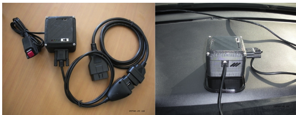
Fig. 1. (a) Automatic data-capture device and (b) its attachment to a car dashboard.
